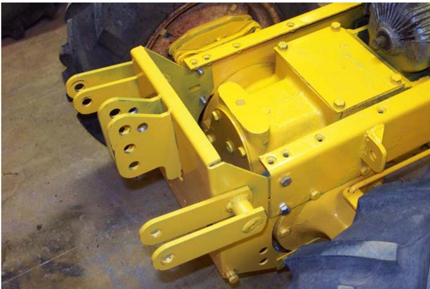
Secure the plate to the frame with the supplied bolts, nuts and lock washers. Use the shorter bolts on the right side of the tractor (if sitting in the seat). Once you get it all in place and movement is accomplished, you may snug down all the bolts in the plate, brackets and axle tubes.
