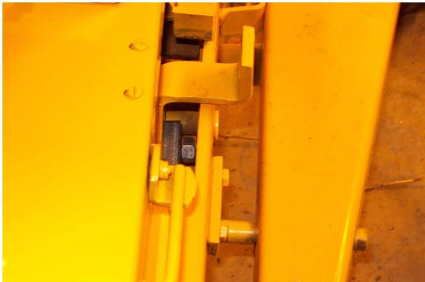
Slide the shaft up to meet the bolt that you inserted earlier. Push the bolt thru now and secure with the supplied nylon lock nut. There is not a lot of room to work, and a 3<sup>rd</sup> hand can come in handy. Tighten the nut snugly and then back off  $\frac{1}{4}$  turn to allow rotation and eliminate binding.
