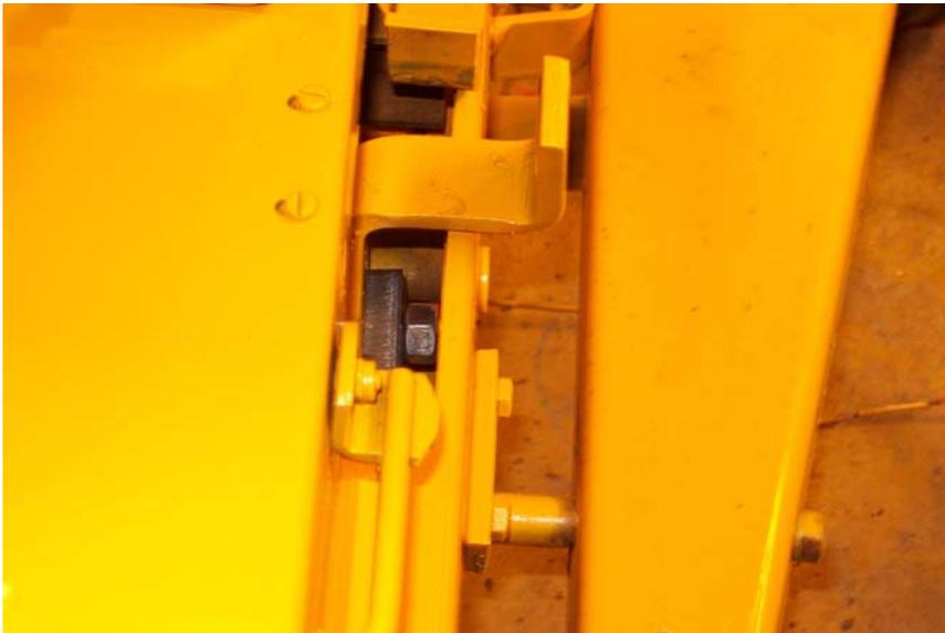
Slide the shaft up to meet the bolt that you inserted earlier. Push the bolt thru now and secure with the supplied nylon lock nut. There is not a lot of room to work, and a 3<sup>rd</sup> hand can come in handy. Tighten the nut snugly and then back off ¼ turn to allow rotation and eliminate binding.
