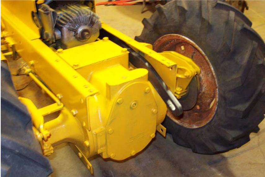
Slide the link shaft thru the frame of the tractor. Watch out for electrical lines.
