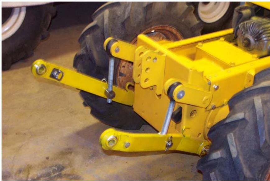
Your 3 point is now basically installed. Check movement by lifting on the arms and by moving the lift that connects to the electric lift or the lift rod. You can adjust the height of the 3 point by moving the furrels up and down on the lift shafts.
