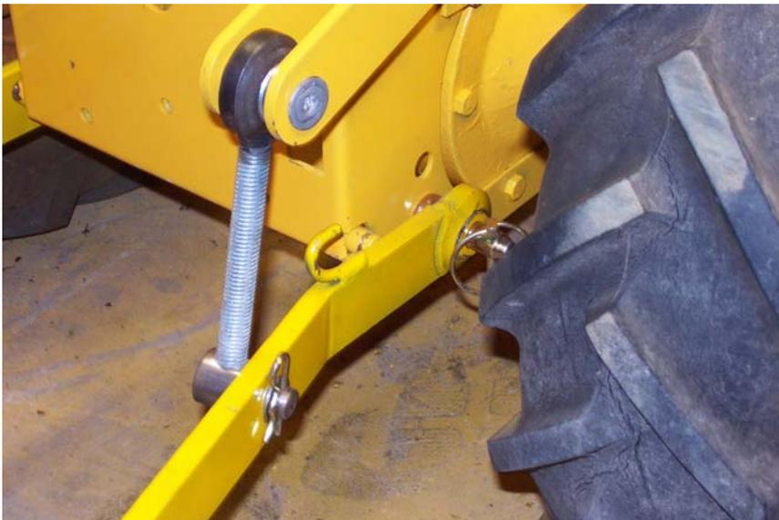
Lubricate all the points that move with oil frequently. The ball sockets will be tight when first put on, but in a short time they will loosen up.
