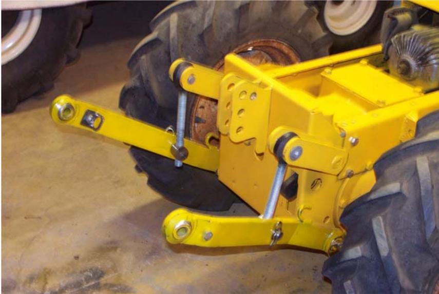
Your 3 point is now basically installed. Check movement by lifting on the arms and by moving the lift that connects to the electric lift or the lift rod. You can adjust the height of the 3 point by moving the furels up and down on the lift shafts.
