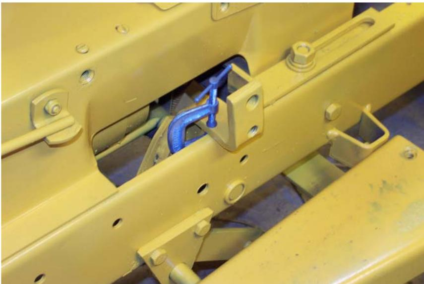
Using a small c-clamp, clamp the lift lever to the short frame lip so that you can drill thru the frame and thru the lift arm. This is the easy way to do it. You could take the whole lift assembly out of your tractor and drill the hole if you do not want an extra hole in your frame.
