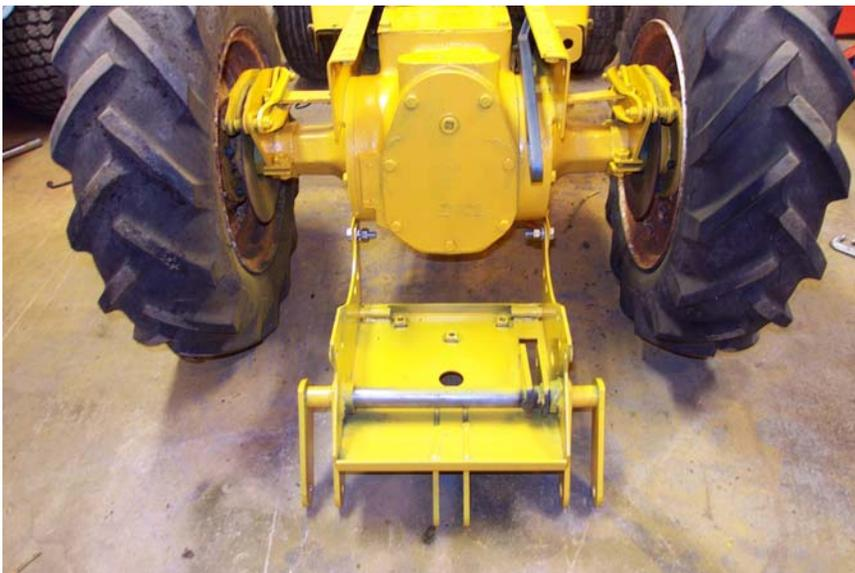
Attach the 3 point plate to the previously installed brackets with the supplied 7/16" bolts, nuts and lock washers. Do not tighten yet – finger tight only.
