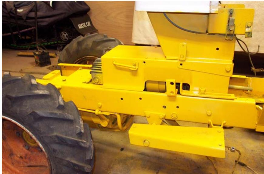
This kit is easiest if the rear fenders and electric lift are off. This is a good time to change the hytran fluid, reseal the rear plate on the differential and any other general work. If you have a hitch on back, remove it and replace the bolts with (3) bolts that are  $\frac{1}{4}$ " shorter.
