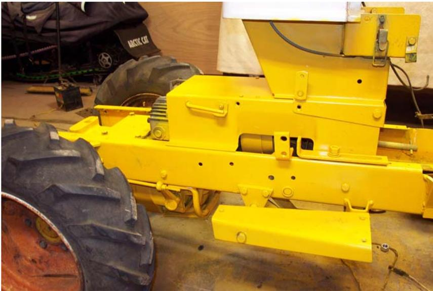
This kit is easiest if the rear fenders and electric lift are off. This is a good time to change the hytran fluid, reseal the rear plate on the differential and any other general work. If you have a hitch on back, remove it and replace the bolts with (3) bolts that are 1/4" shorter.
