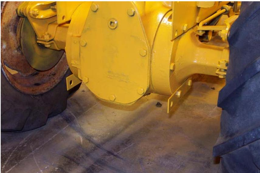
Attach the rear brackets to the axle housings by taking out the existing lower 2 bolts and putting the bracket over them and re-inserting them. Do not tighten them tight yet – just finger tight. The 2 holes that bolt to the tractor should be towards the top and the larger hole to the back of the bracket should be down.
