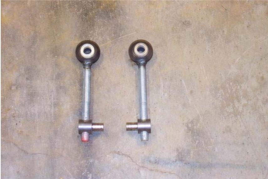
Assemble the lift links and furlers as shown. Lubricate the threads in the furlers with grease prior to assembly and through out the life of the lift.
