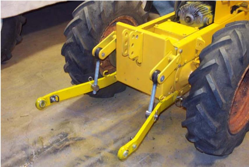
Attach the lift arms to the tractor, with the supplied pins.
