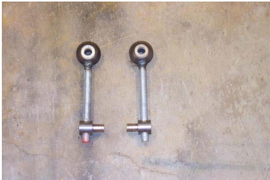
Assemble the lift links and furrels as shown. Lubricate the threads in the furrels with grease prior to assembly and through out the life of the lift.
